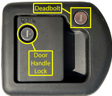
The orientation of the latch assembly shown above may be inverted on your trailer, depending on the direction the door opens.
