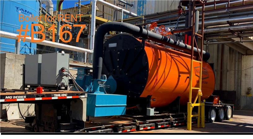
Hurst Series 400, 900 HP Steam Boiler 900 HP - 150 psig Steam Skid-Mounted Boiler
