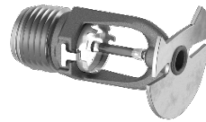
Window Sprinkler Quick Response Glass Bulb Horizontal Sidewall (Specific Application) SIN: VK962 K Factor: 5.6 (81) Thread Size: 1/2 inch NPT Base Part #: 23834
