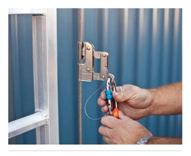
**Step 7**Check the shuttle is functioning correctly and all carabiner screw gates are secure.
