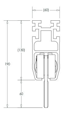
15kN RATED FOR FALL ARREST APPLICATIONS
