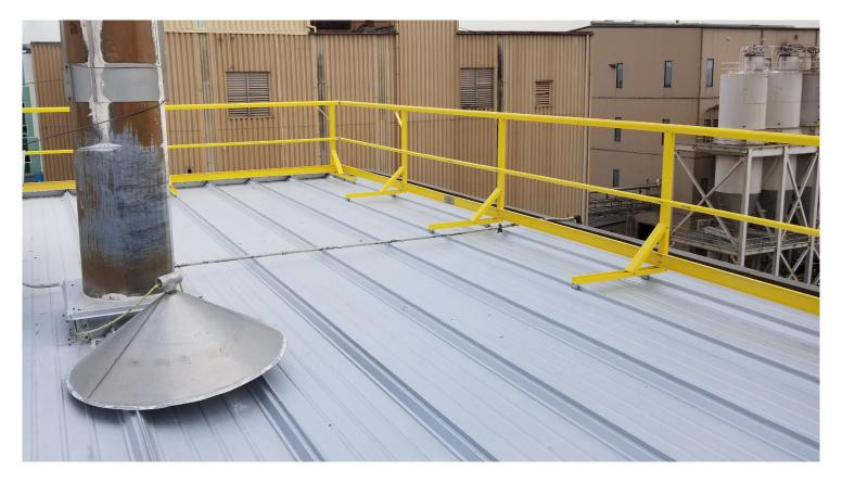
GR32 Metal Roof Mount Guardrail is designed for metal roofs including R panel and standing seam systems. The GR32 system can either be fastened down with self-sealing rivets to the metal deck or with non-penetrating clamps to suit the standing seam profile. Roof guardrail systems can be purchased by simply selecting the kit length(s) required, the number of corner kits, wall termination kits and ladder connection hardware kits. GR32 guardrail is simple and quick to install.
