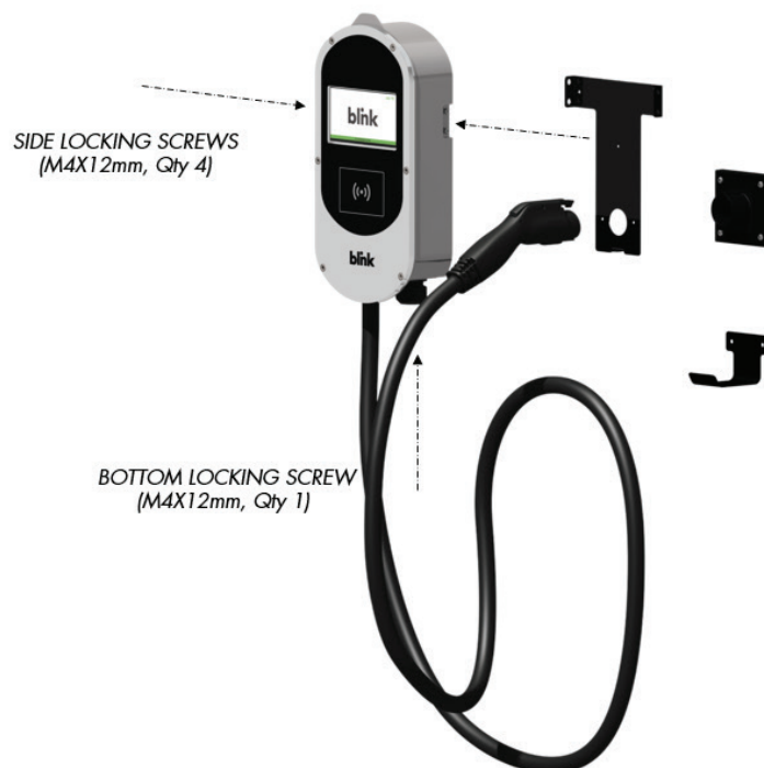
Fig. 13 – Head Unit mounting to Wall Bracket
