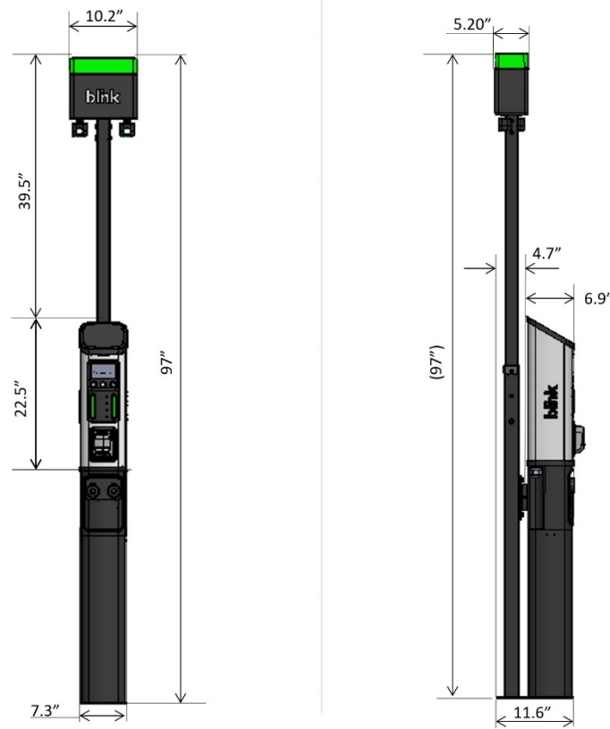
Fig. 6 – Series 8 – ISO charger with pedestal and cable management system
