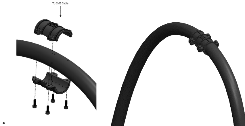
Fig. 53 – Installing CMS cable clamp
