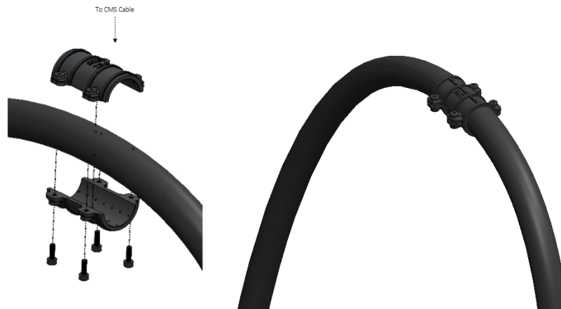
Fig. 46 – Installing CMS cable clamp
