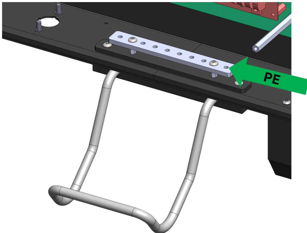
Fig. 51 – Input Ground wire connection
