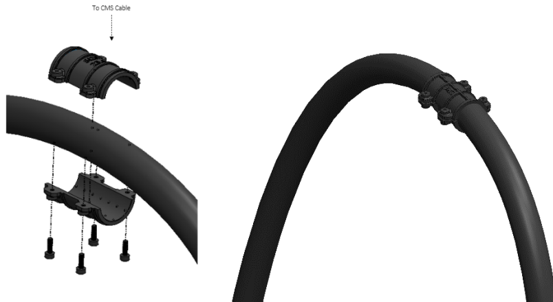
Fig. 53 – Installing CMS cable clamp
