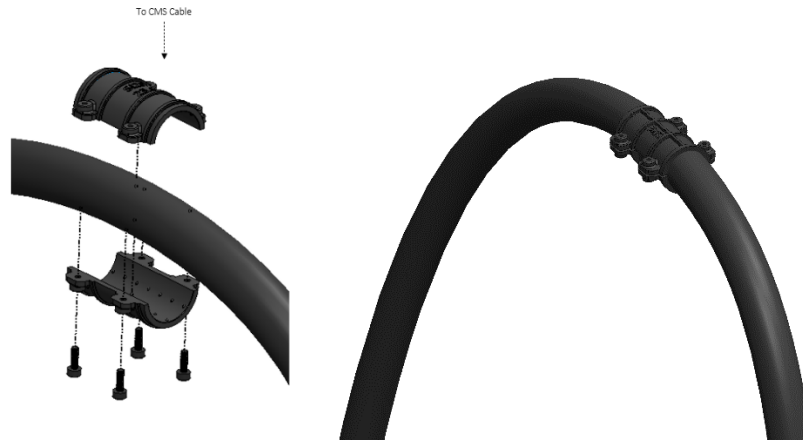
Fig. 46 – Installing CMS cable clamp
