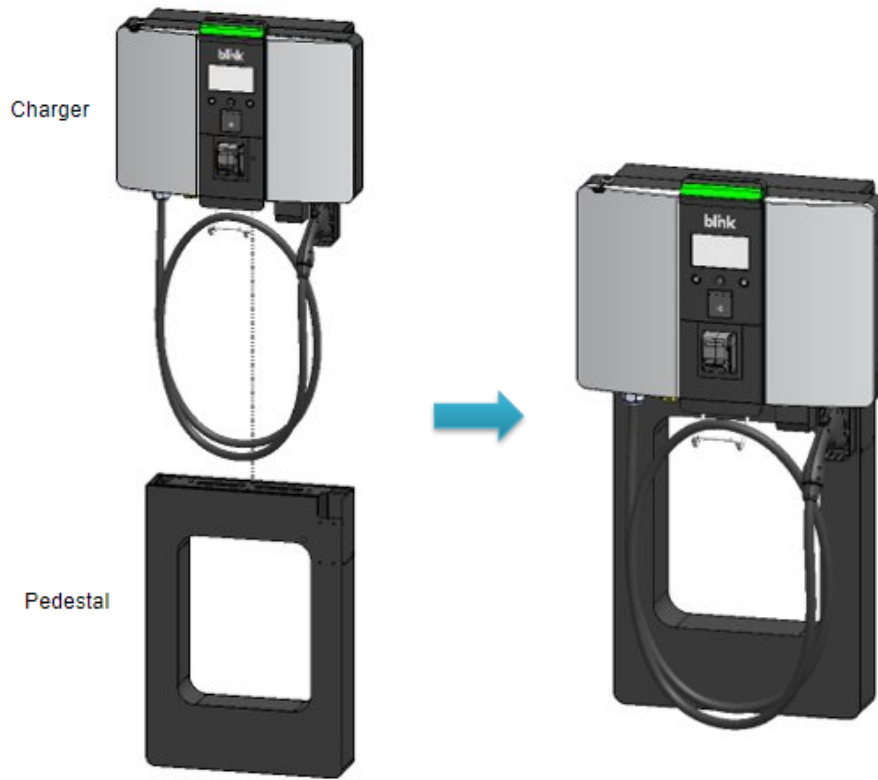
Fig. 25 – Mounting Head Unit on Pedestal
