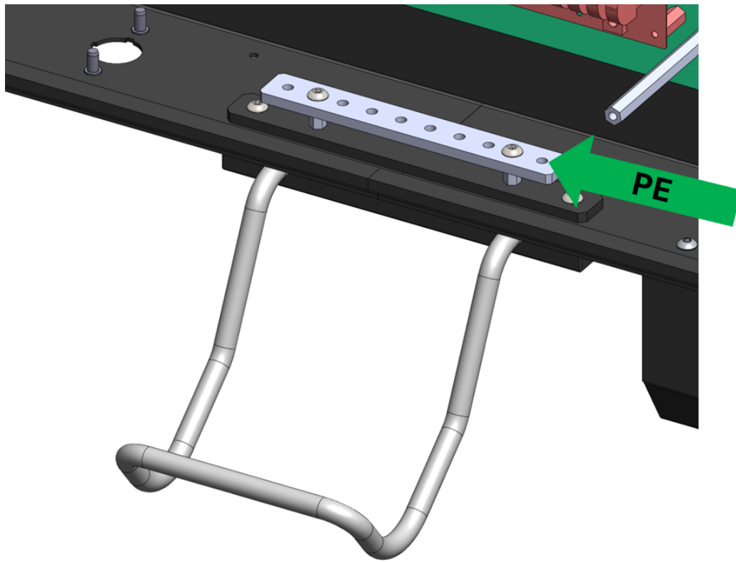
Fig. 50 – Input Ground wire connection
