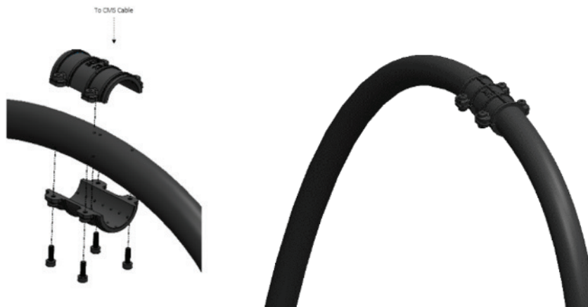
Fig. 22 – Installing CMS cable clamp
