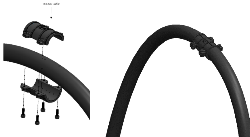
Fig. 46 – Installing CMS cable clamp
