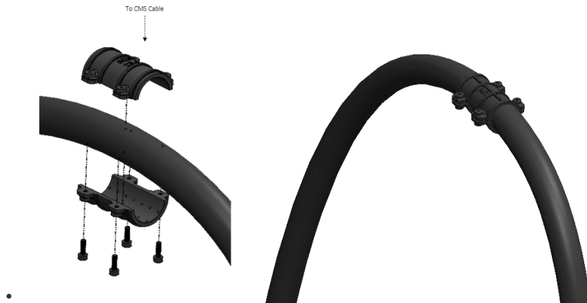
Fig. 53 – Installing CMS cable clamp
