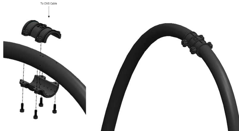
Fig. 53 – Installing CMS cable clamp
