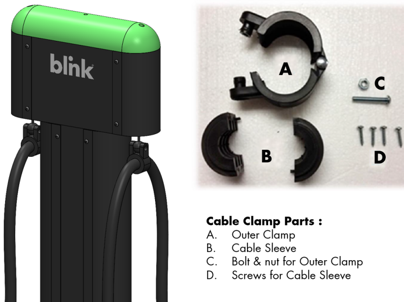
Fig. A-14 – Cable clamp assembly
